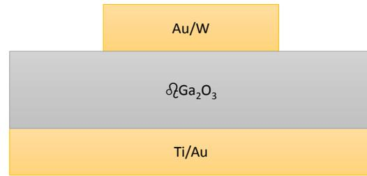
**Fig. 8.** Cross-section of the vertical Schottky rectifier with W contacts, adapted from [58].
